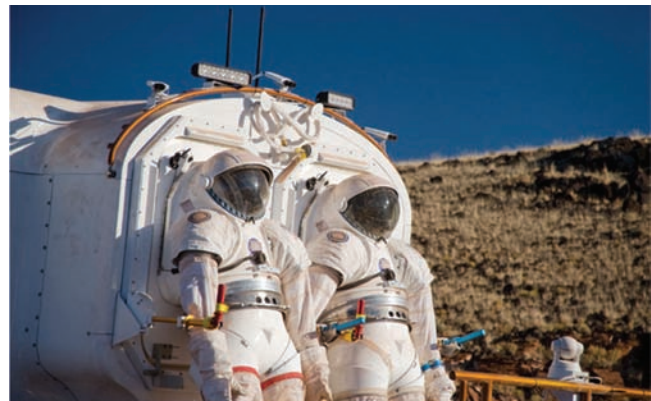
Fig. 2. Aft bulkhead mockup with Mark III mockup suits attached to suit ports.
